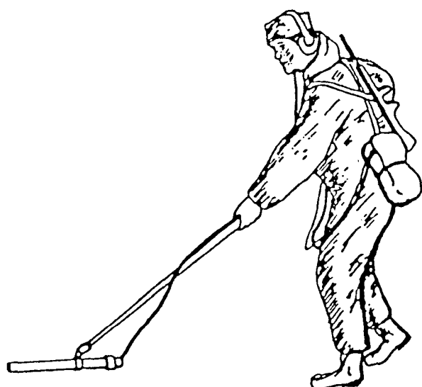
Figure C-8. IMP (portable mine detector)
